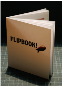
FIGURE 17.25 The final saddle-stitch book has staples on the spine. You may want to trim the outer edges of the pages once the book is assembled.
